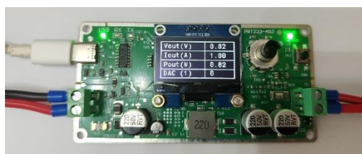
Figure 14 PBT223-ADJ DAC 模式 = 0
