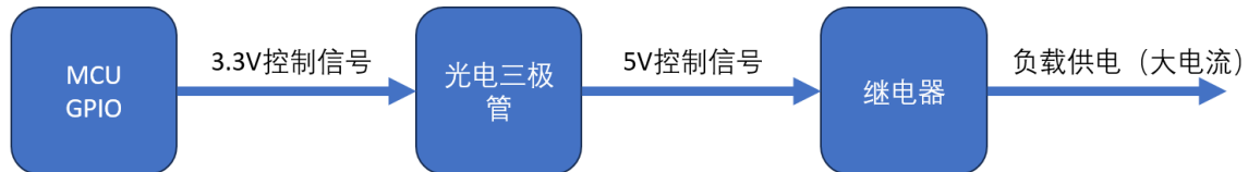
Figure 14 MCU 与继电器光耦隔离
